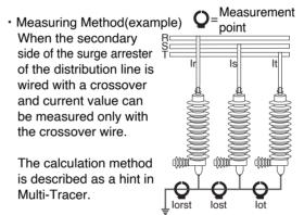
When measuring on the secondary side of the testing surge arrester at the substations or distribution lines.
